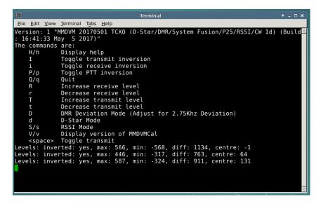
To calibrate, we press "D" to enter DMR Deviation Mode. A simple sine wave tone at 1200Hz is sent here. Either you are now the happy owner of a measuring station, or you simply have an RTL-SDR stick.
