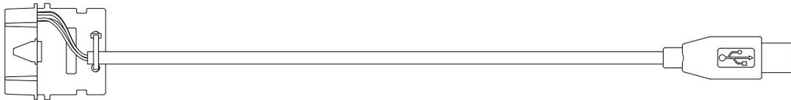
Figure 2-1. Mobile & Repeater Rear Programming Cable PMKN4010\_
